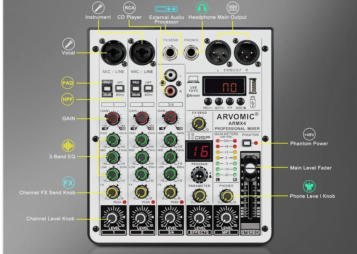
Figure 2: Labeled diagram of the ARMX-4 mixer's controls. This image highlights key components such as MIC/LINE inputs, PAD and HPF buttons, GAIN controls, 3-Band EQ (HIGH, MID, LOW), FX SEND knobs, Channel LEVEL knobs, +48V Phantom Power switch, Main Fader, and Phone Level knob, providing a clear guide to each function.
