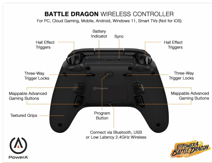
Back view of the controller highlighting the Battery Indicator, Sync Button, Hall Effect Triggers, Three-Way Trigger Locks, Mappable Advanced Gaming Buttons, Program Button, and Textured Grips. Also shows connection options via Bluetooth, USB, or 2.4GHz Wireless.
