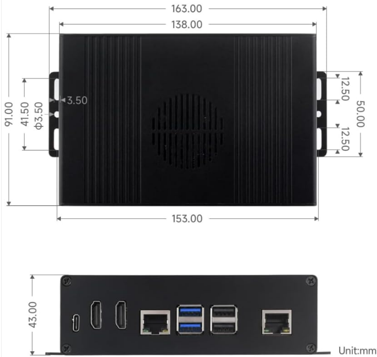
Figure 8.1: Outline dimensions of the waveshare Mini-Computer Kit. This technical drawing provides precise measurements of the assembled case in millimeters.
