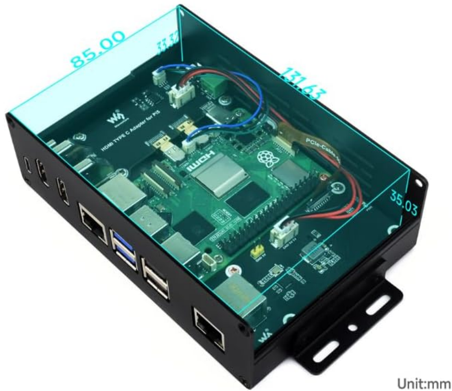
Figure 2.5: Internal space and expandability. This image shows the internal dimensions of the case, indicating ample room for the Raspberry Pi 5 and additional HATs, with measurements in millimeters.
