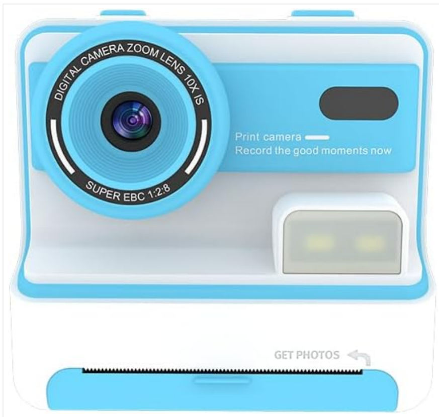
Image 4.1: Front view of the camera, highlighting the lens, flash, and paper output slot.
