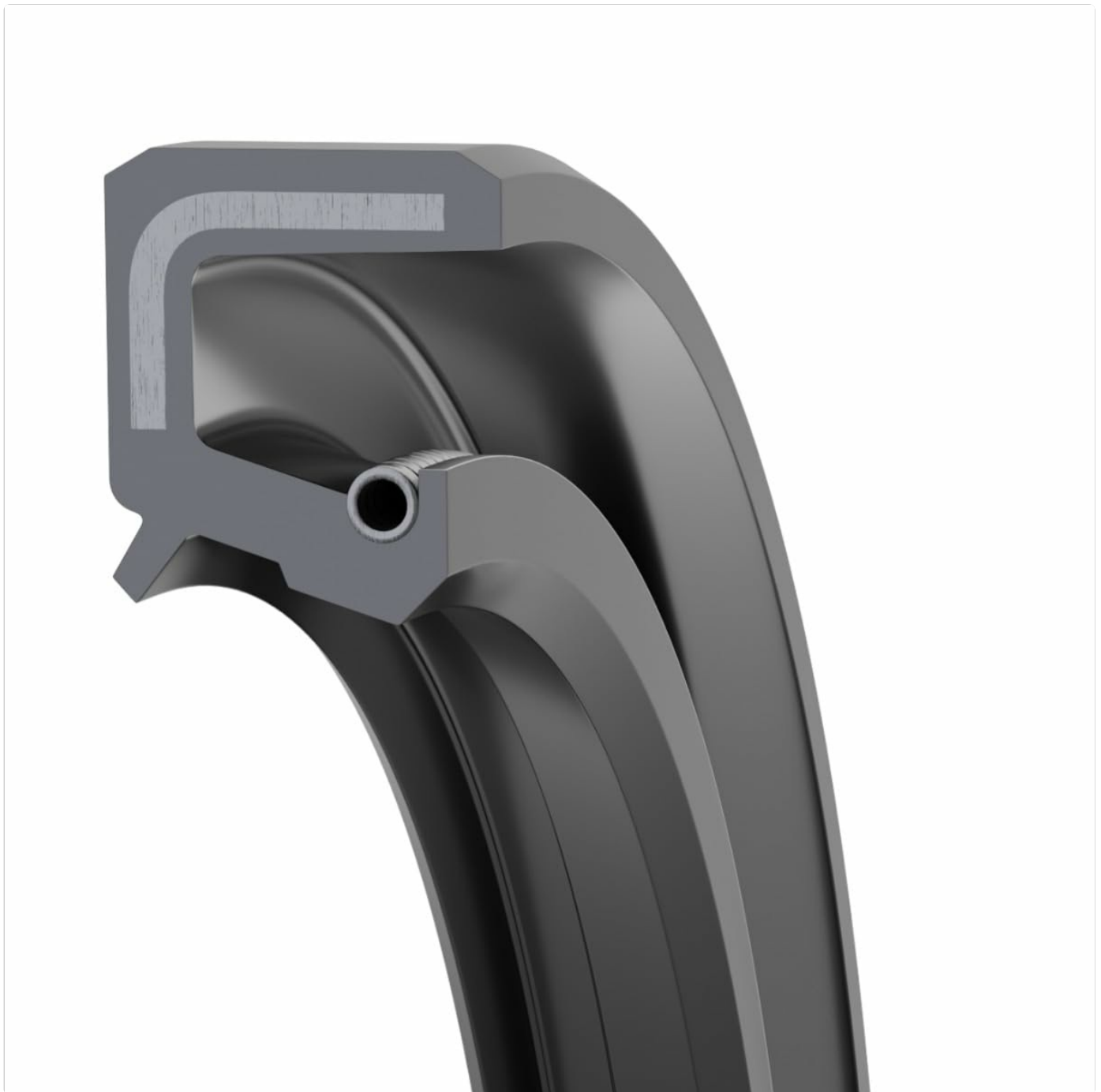
Figure 2.1: Cross-section of the NMD TC Rotary Shaft Oil/Dust Seal. This image displays a detailed cross-section of the TC rotary shaft oil seal. It highlights the main sealing lip, the auxiliary dust lip, and the garter spring which provides radial force to maintain contact with the shaft. The robust design ensures effective sealing against lubricants and protection from contaminants.
