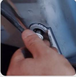
1. Loosen driver/passenger hood hinge bolts and washers and make clearance for the brackets.
