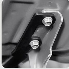
2. Insert the brackets in between hood hinge and bolts.
