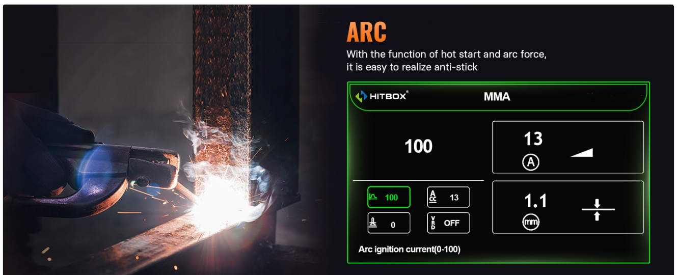
Figure 6.1.3: Stick (MMA) mode display.
