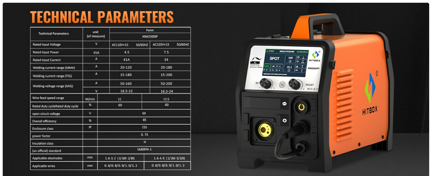
Figure 9.1: Technical Parameters for HIM250DPP.
