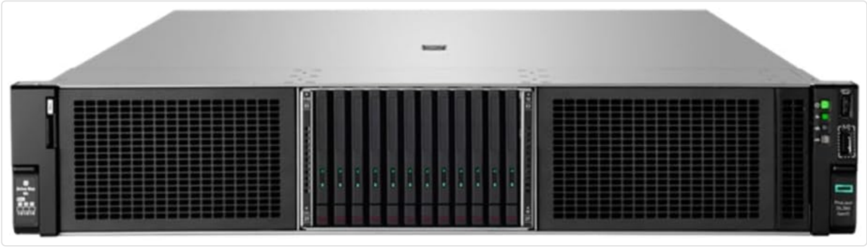
Figure 4.5: Front view of the HPE ProLiant DL380 Gen11 server, showing drive bays, control panel, and power button.
