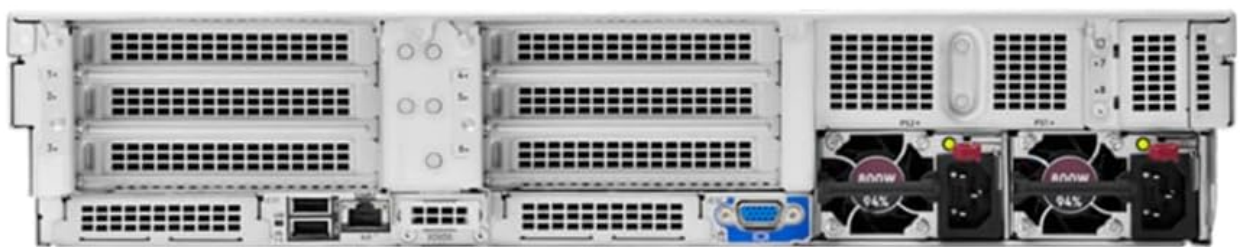
Figure 4.4: Rear view of the HPE ProLiant DL380 Gen11 server, highlighting power supply bays, network ports, and other I/O connections.
