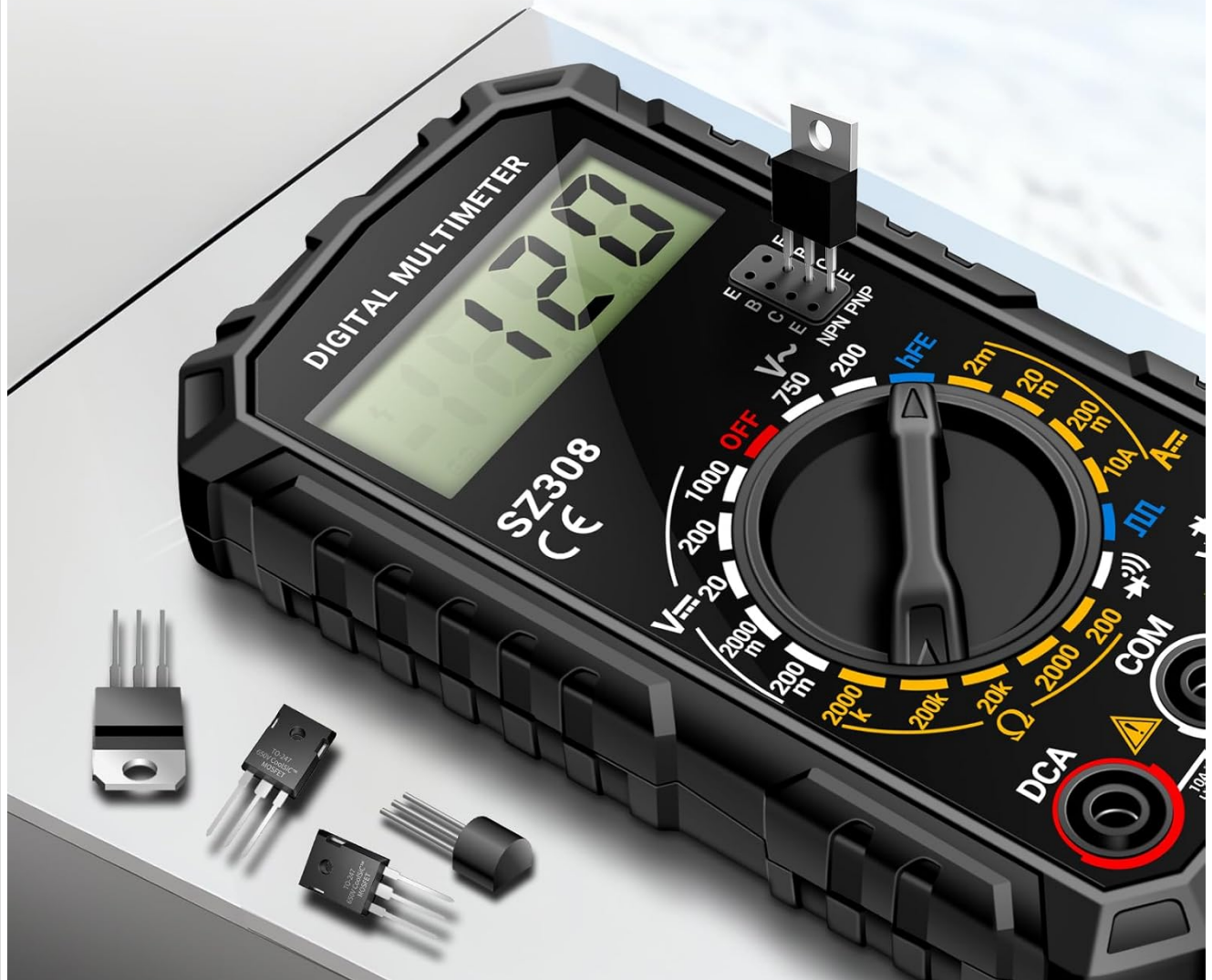
Figure 6: Performing an hFE Triode test.
