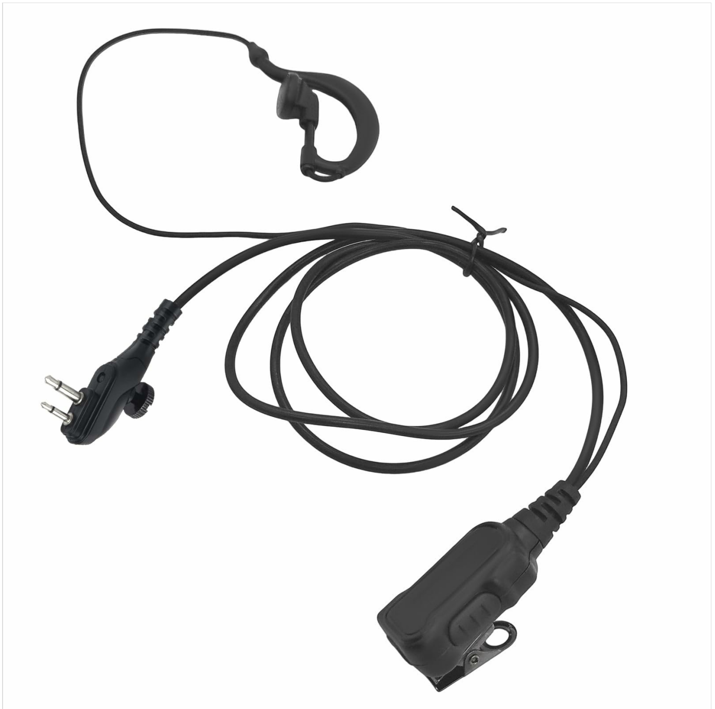
Figure 1: The PTT button and microphone unit, featuring a sturdy clip for attachment to clothing.
