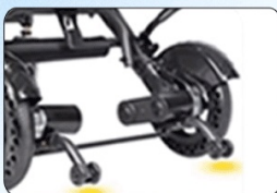
Figure 4.3: The New Smart Brake system automatically parks the wheelchair even without power, featuring reverse anti-rollback wheels and dual handbrakes for comprehensive protection.
