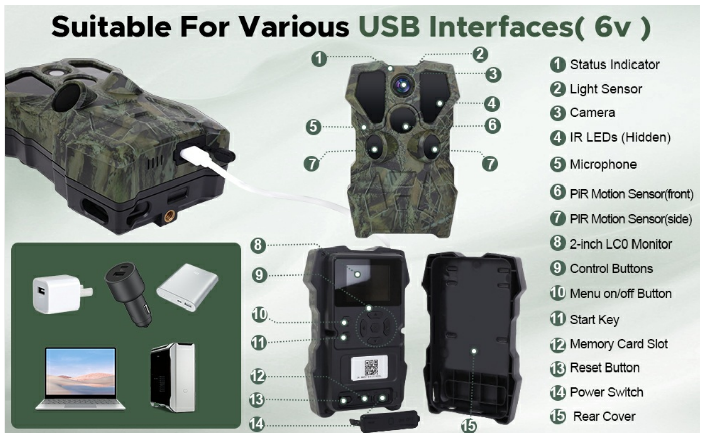
Image 3.1: Detailed diagram of the MKEOLGE X1 Trail Camera's external and internal components.
