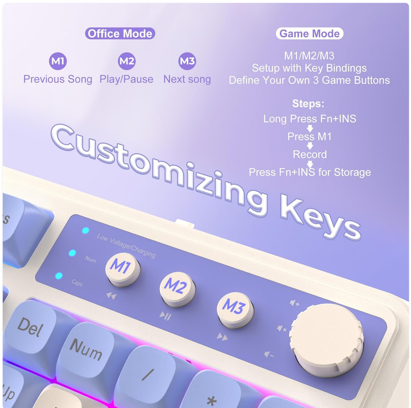
Figure 5: Macro customization for M1/M2/M3 buttons.
