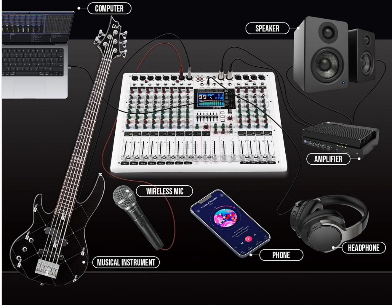
Figure 4: Example of multiple device interconnection, illustrating how to connect a computer, musical instruments (guitar), microphones (wireless mic), mobile phone, headphones, amplifier, and speakers to the mixer.
