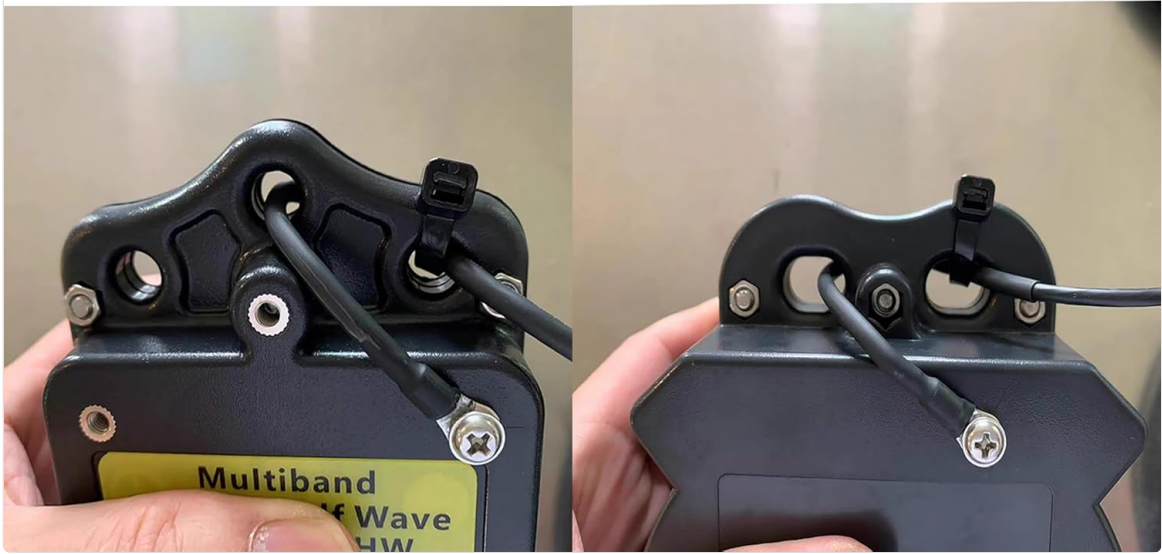
Image: Close-up view demonstrating how to connect the antenna wire to the balun's terminals for both 4-band and 8-band configurations.
