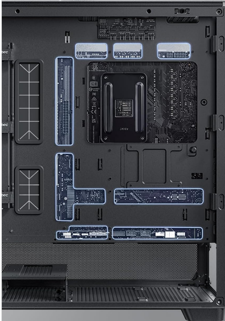
Figure 4: Illustration of back-connect motherboard support, enabling hidden cable routing for improved aesthetics and airflow.
