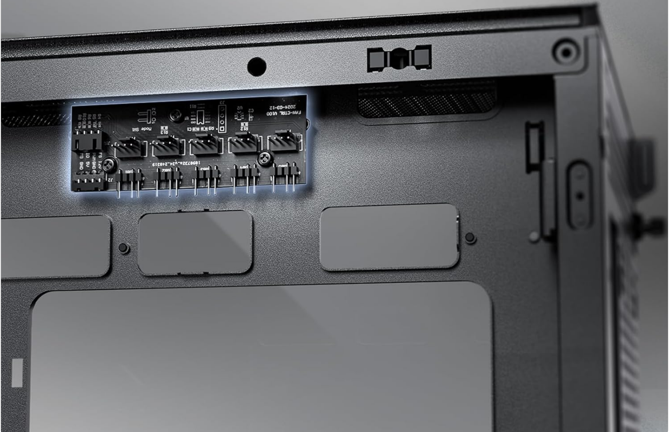
Figure 9: The integrated ARGB & PWM fan control hub, simplifying fan management and synchronization with the motherboard.
