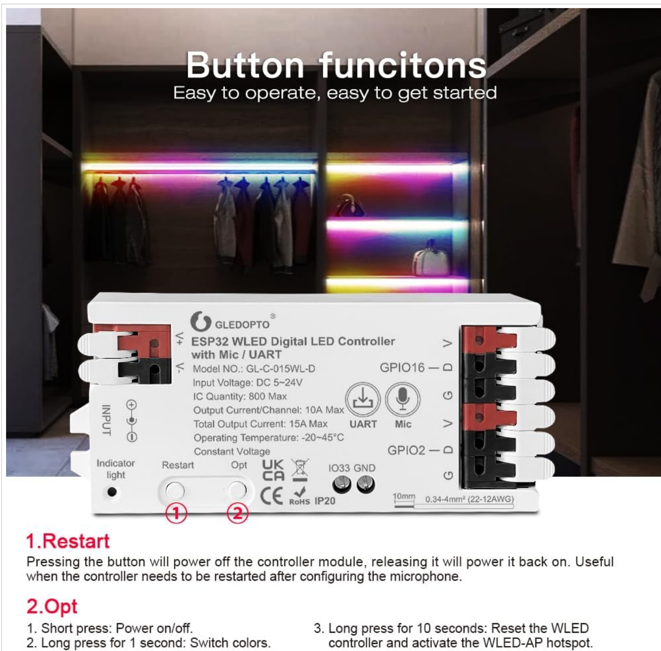
Figure 4: Button Functions. This close-up image of the GLEDOPTO controller highlights the 'Restart' and 'Opt' buttons. It details that the 'Restart' button powers off and on the controller, useful for restarting after microphone configuration. The 'Opt' button has functions for short press (power on/off), long press for 1 second (switch colors), and long press for 10 seconds (reset WLED controller and activate WLED-AP hotspot).
