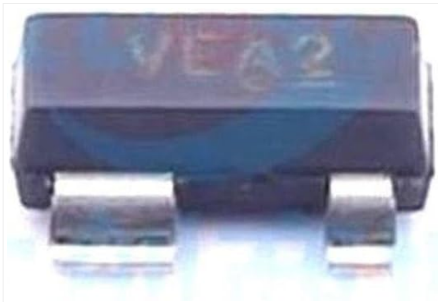
Figure 1: Close-up view of the CAT811STBI-GT3 chip. This image shows the compact SOT-143-4 package with its four pins, highlighting the component's small size and surface-mount design.
