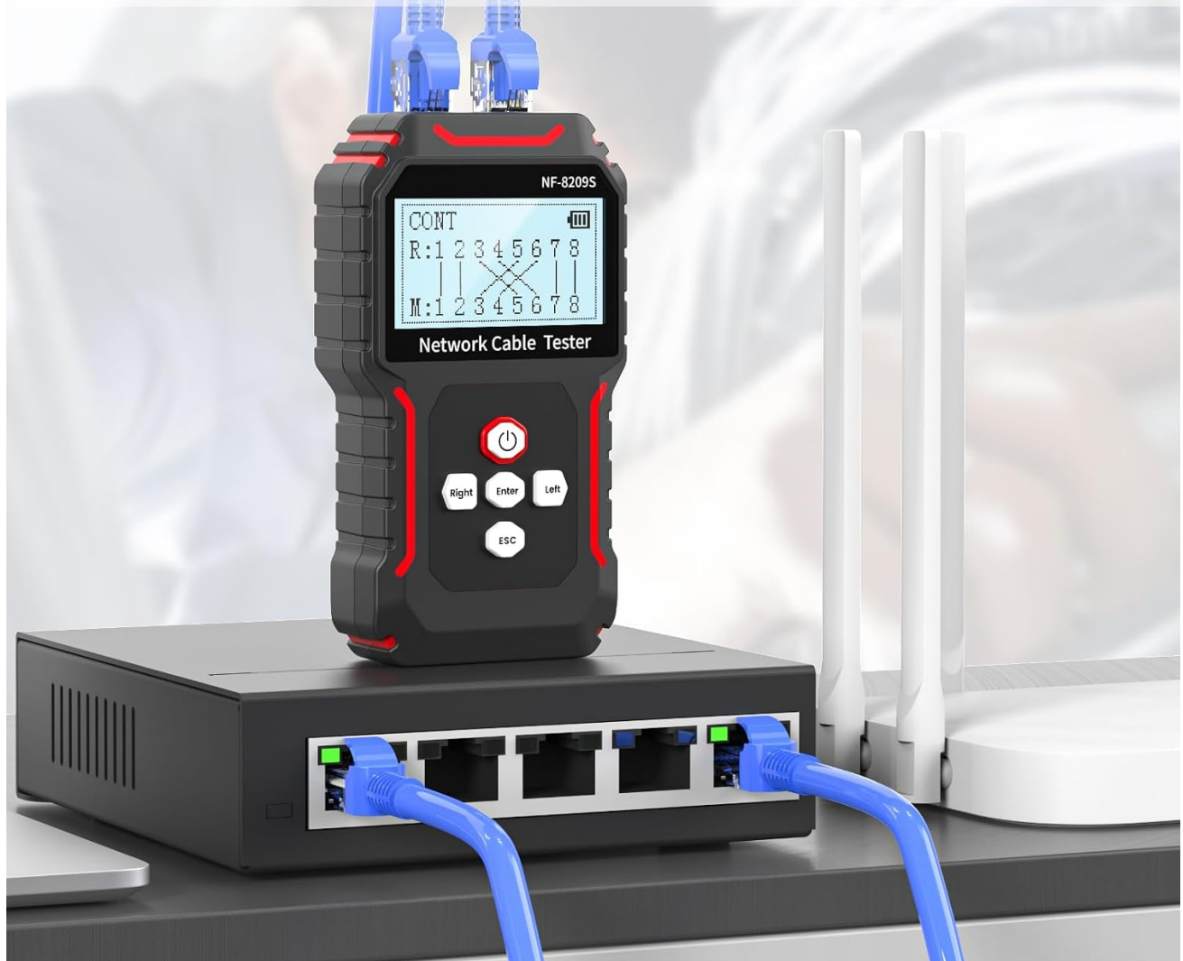
Figure 5: Cable fault testing setup, detecting shorts, opens, crosses, and breaks in network cables.
