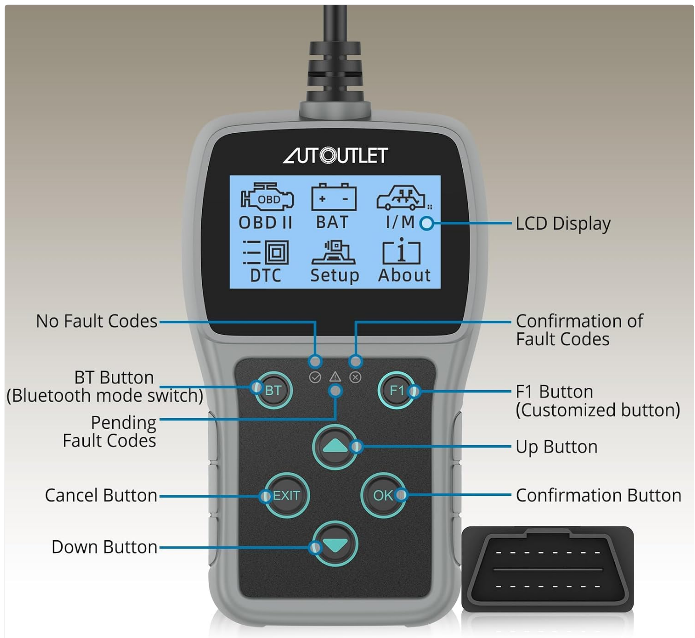
Image: Detailed diagram of the diagnostic tool showing the LCD Display, BT Button (Bluetooth mode switch), F1 Button (Customized button), Up Button, Down Button, EXIT (Cancel Button), and OK (Confirmation Button). The OBDII connector is also visible.
