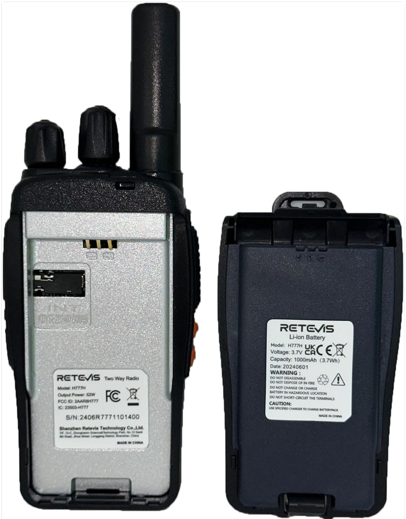
Image: View of the back of the Retevis H-777H walkie talkie with its battery pack detached, showing the connection points.
