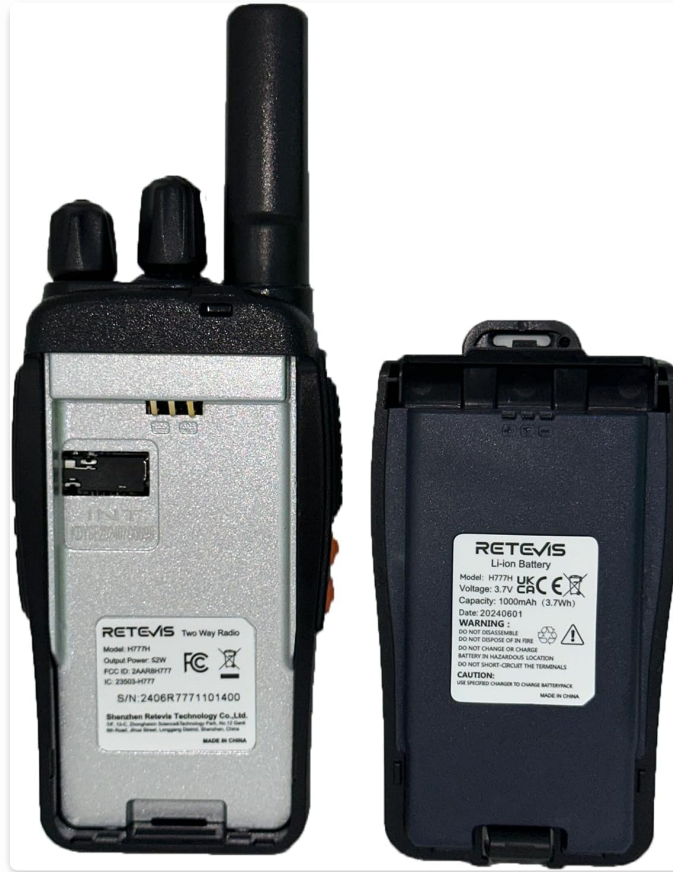
Image 4.1: Battery Compartment and Battery
