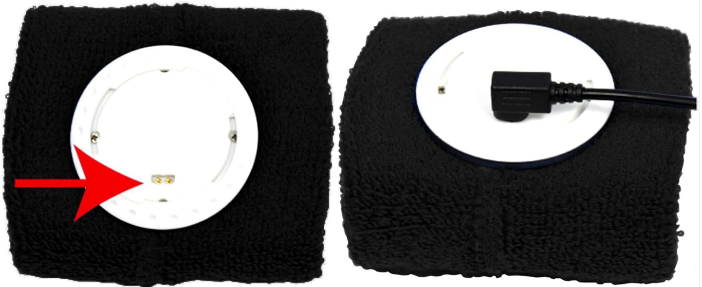
Figure 3: Instructions for charging the Coolfire watch module using the provided USB cable.
