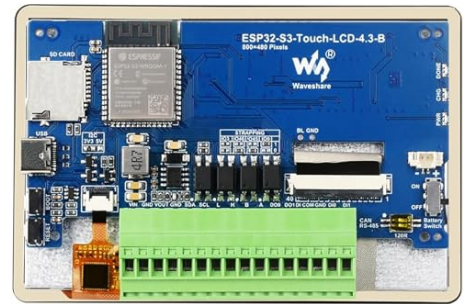
Figure 3: Detailed view of the ESP32-S3-Touch-LCD-4.3B board components.
