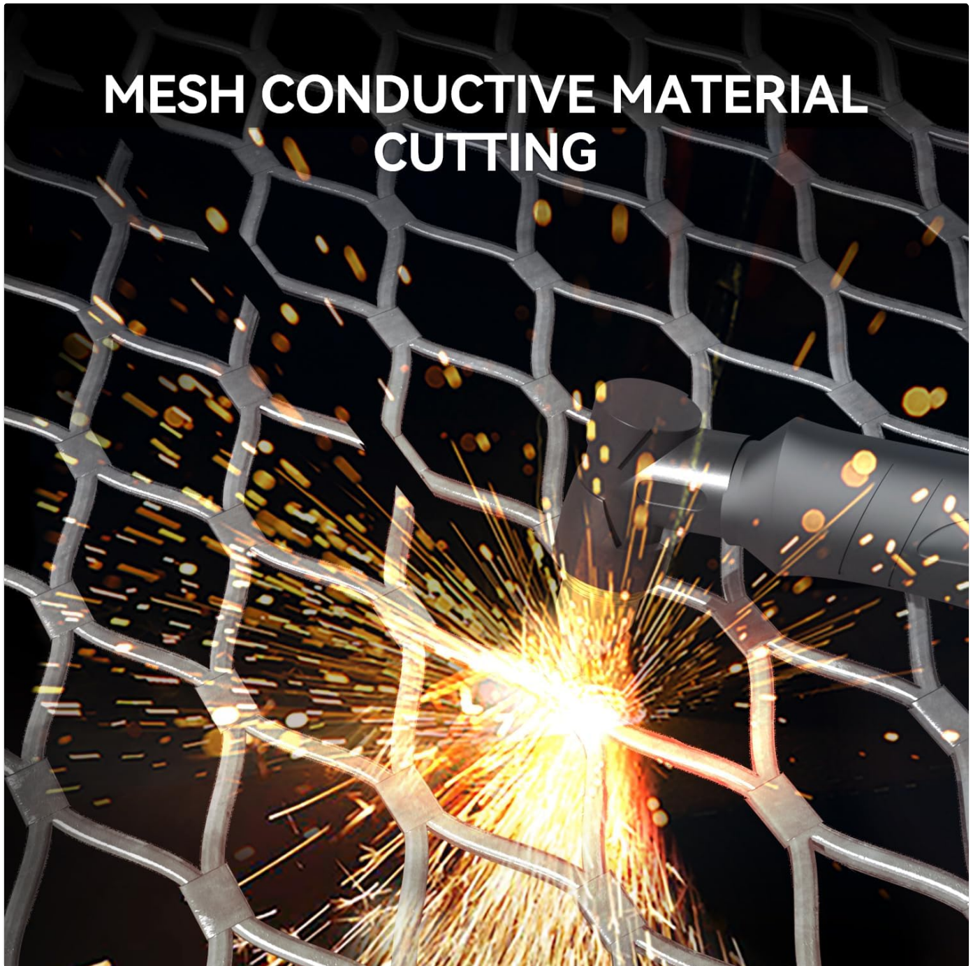
Figure 4.2: Example of plasma cutting mesh material.
