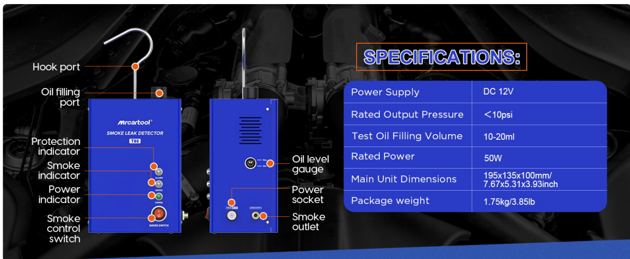
Image 4.1: Detailed specifications and labeled parts of the T80 unit.
