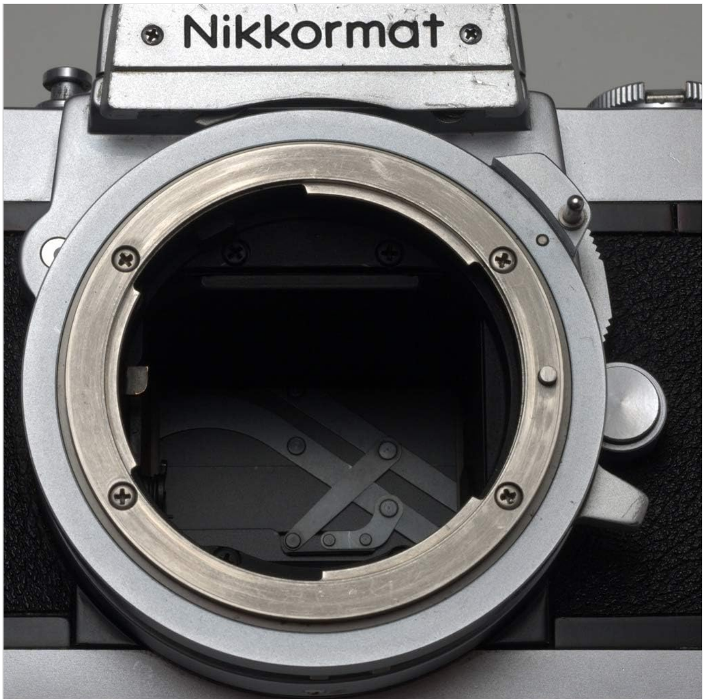
Figure 4: Detailed view of the Nikomat FTN's lens mount and internal mirror box.
