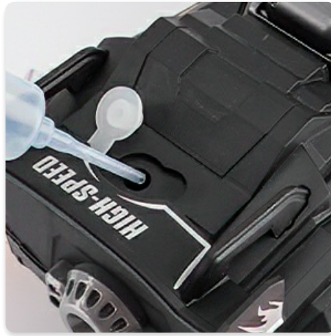
Figure 3: Water injection port for the spray feature.
