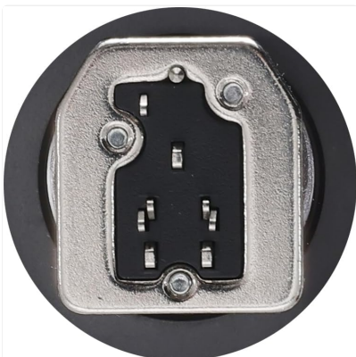
Figure 3.3: This close-up image details the hot shoe connection pins of the JINBEI
