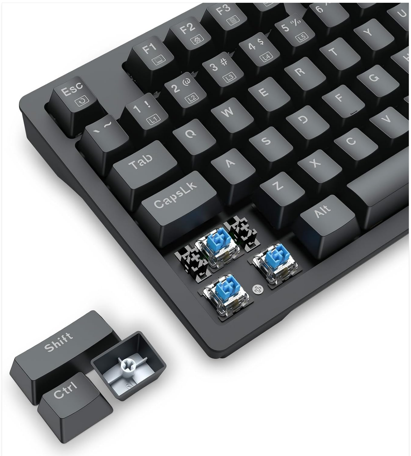
Image: A close-up view of the Redragon K679 keyboard with several keycaps removed, illustrating the hot-swappable mechanical switches.
