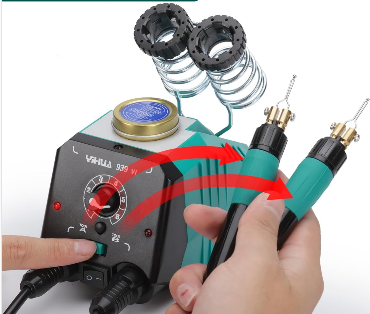
Figure 6.2: Using the A/B toggle switch to select the active pen.
