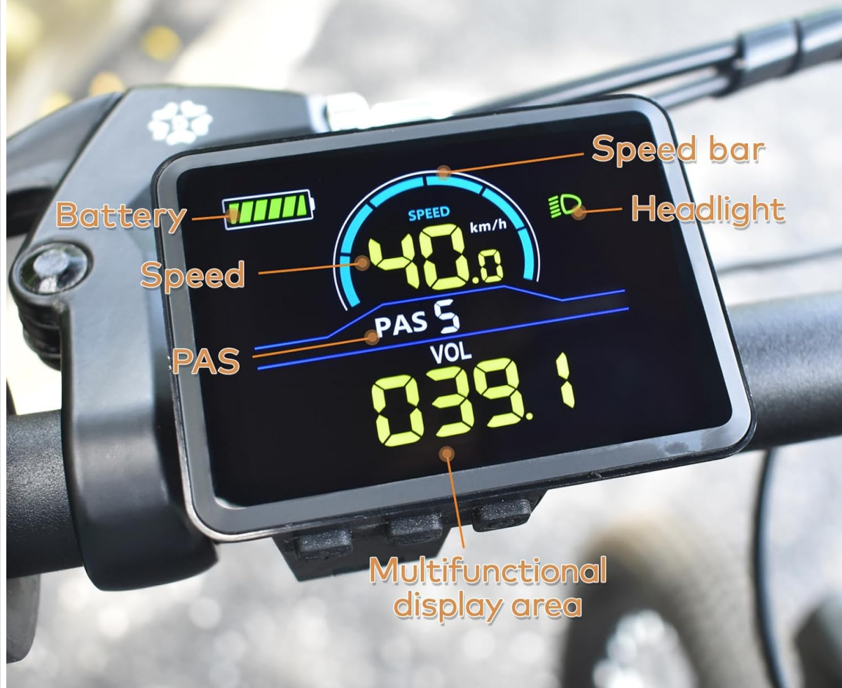
Image: The Mcezy P5C Ebike LCD Display illustrating key metrics such as speed, battery level, Pedal Assist System (PAS) level, and voltage.
