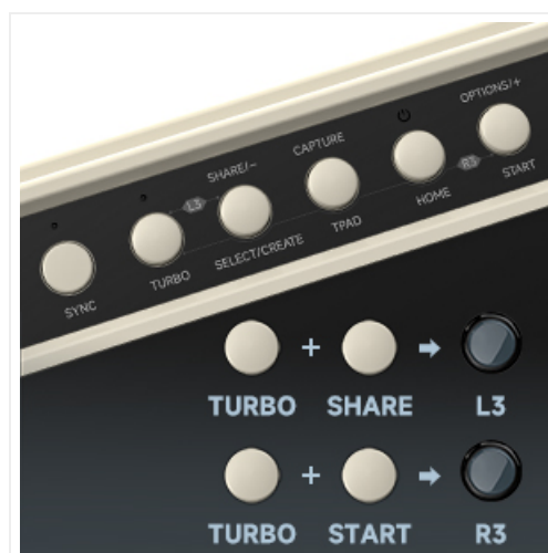
Image: A diagram illustrating the button combinations for activating L3 (TURBO + SHARE) and R3 (TURBO + START) on the F700 Elite.
