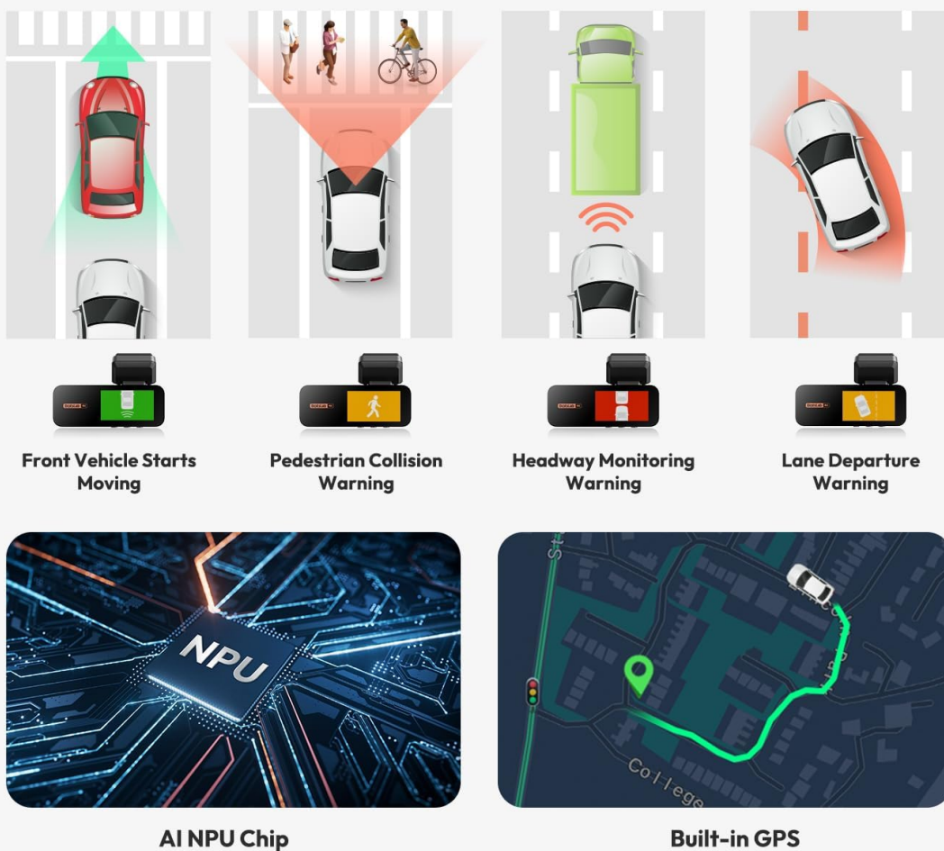
Figure 5.1: Visual representation of ADAS alerts and the AI NPU chip.
