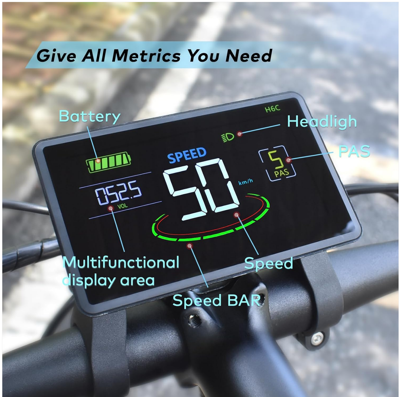
Figure 3.1: Display Metrics Overview. This image highlights the different data points shown on the H6C display, including battery level, speed, PAS level, headlight indicator, and a multifunctional display area.
