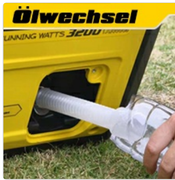
Image 8: Performing an engine oil change.
