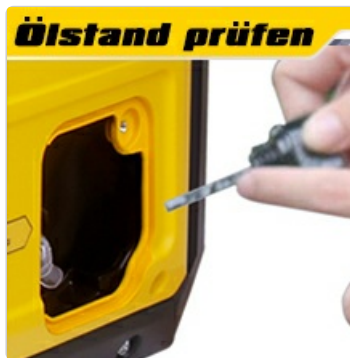
Image 3: Checking the engine oil level using the dipstick.
