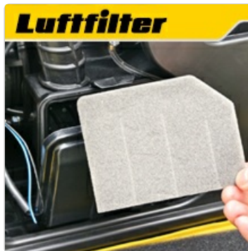
Image 9: Inspecting and cleaning the air filter.
