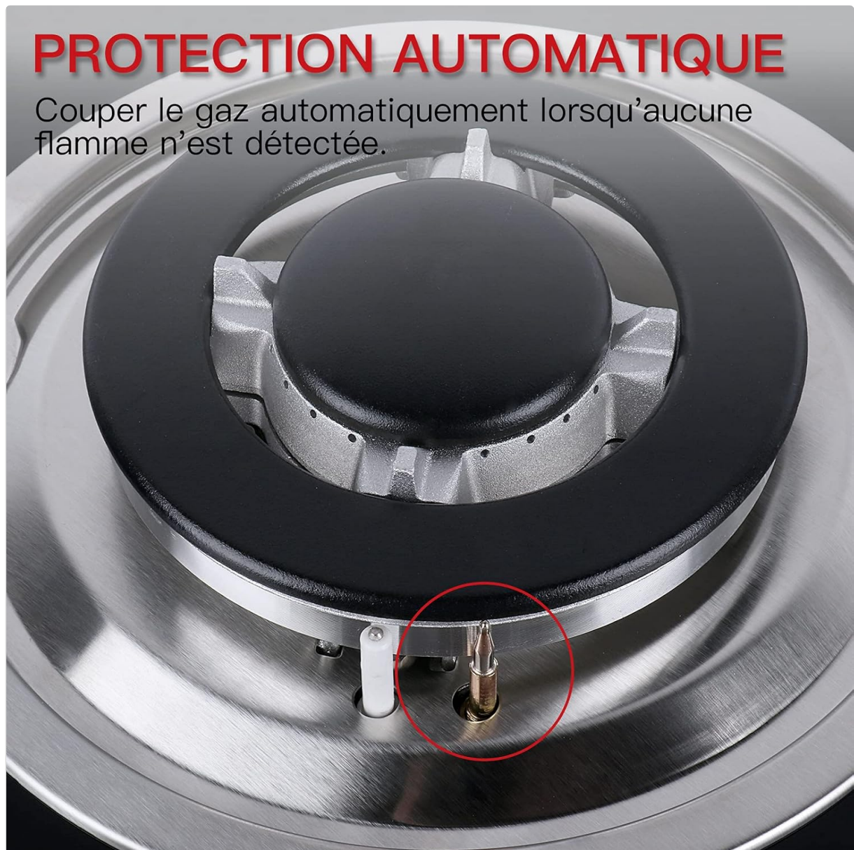
Figure 7: A detailed view of a gas burner, highlighting the thermocouple (circled in red). This component is part of the automatic protection system, designed to cut off the gas supply if no flame is detected, enhancing safety.
