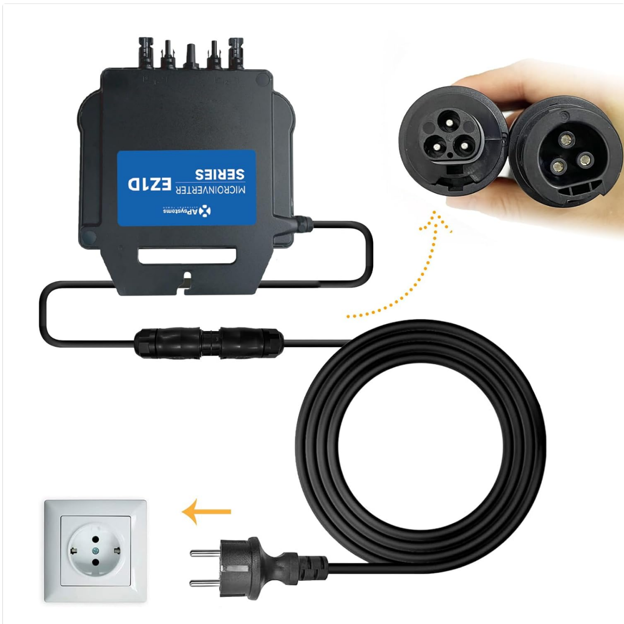
Figure 3: Connection diagram illustrating how the micro-inverter connects to a standard household socket via the Betteri BC01 connector and Schuko plug.
