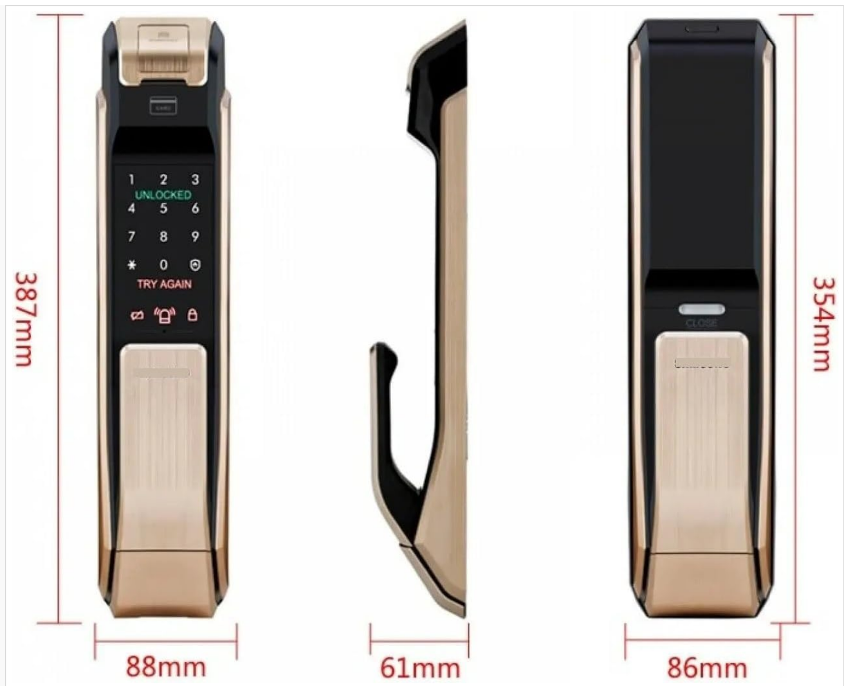
Figure 1: Product Dimensions. This image illustrates the precise measurements of the lock, including its height (387mm and 354mm for different sections), front width (88mm), side depth (61mm), and rear width (86mm), crucial for proper door preparation.
