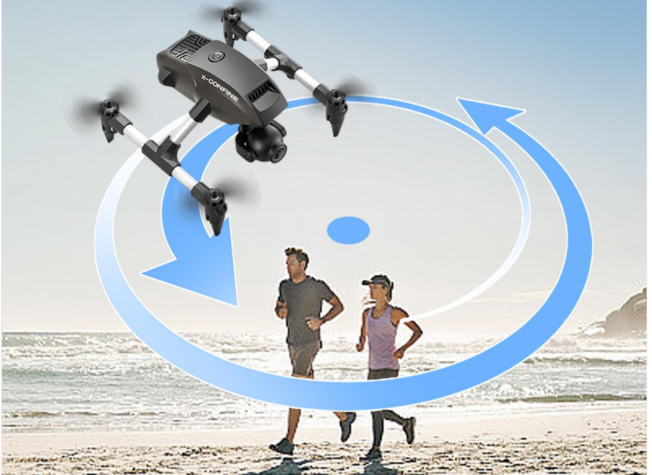
Image: A drone flying in a circular path around two individuals jogging on a beach, illustrating the Circle Flight mode.
