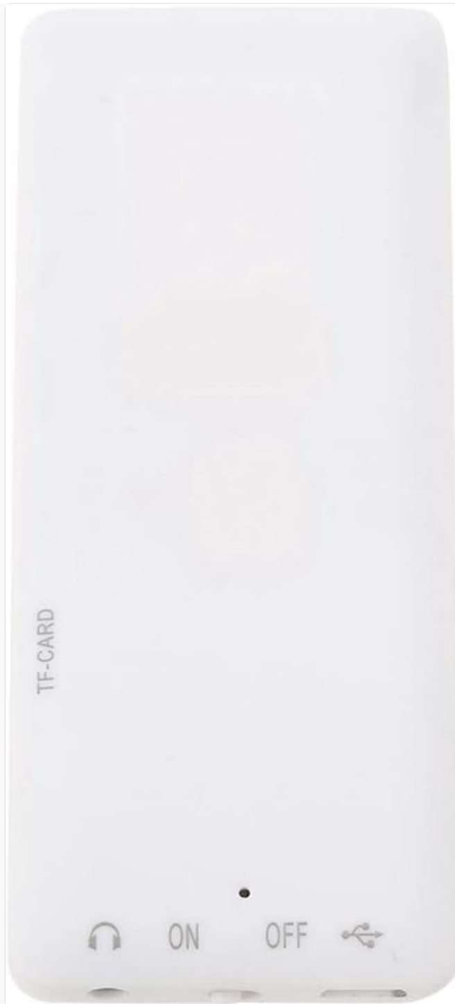
Image: The bottom edge of the MP3 player, showing the TF-CARD slot, ON/OFF switch, headphone jack, and USB port.
