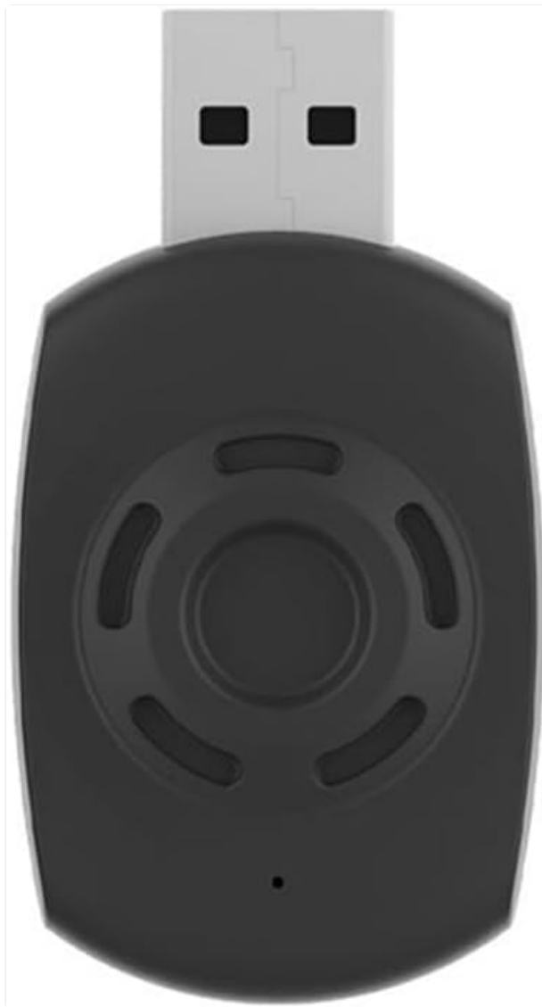
Figure 2.1: Top view of the XGFTHG Acodo Wireless Adapter.
