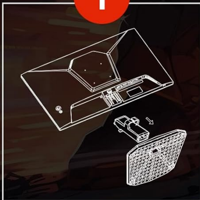
Figure 3: Step-by-step guide for the tool-free installation of the monitor stand, demonstrating how to attach the base to the neck and then to the monitor.
