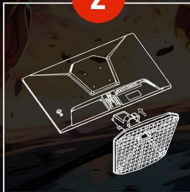
Figure 3: Step-by-step guide for the tool-free installation of the monitor stand, demonstrating how to attach the base to the neck and then to the monitor.
