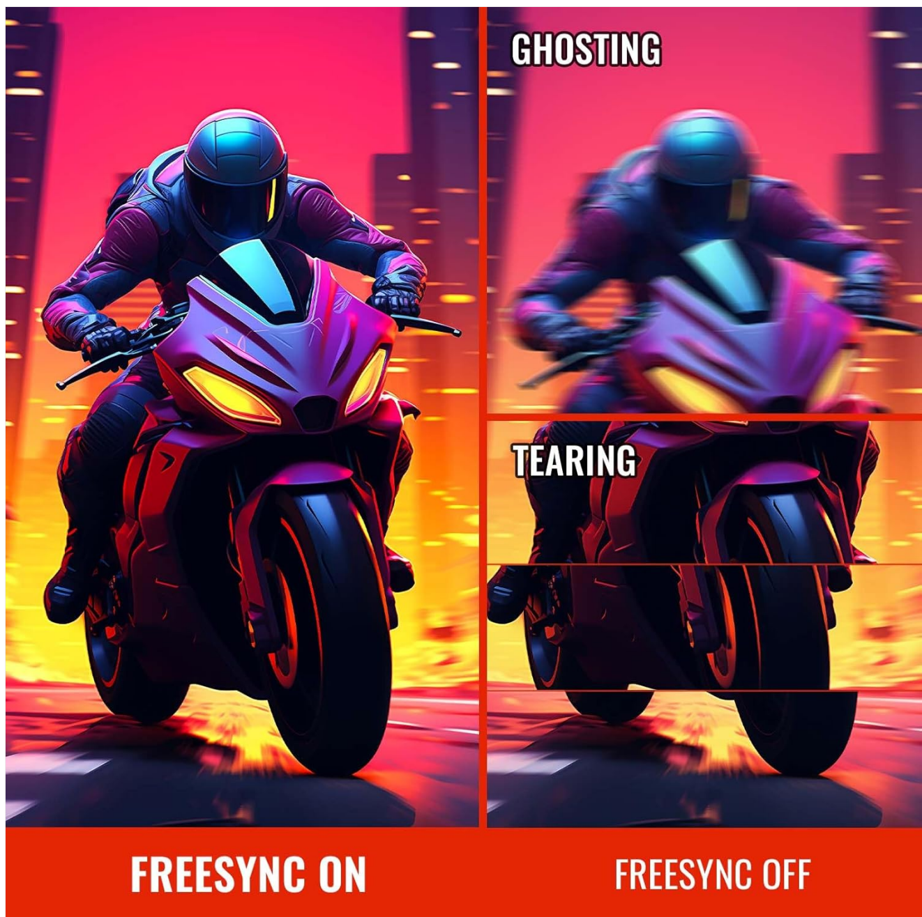
Figure 9: Illustrates how FreeSync technology prevents screen ghosting and tearing, providing a smoother visual experience compared to when FreeSync is off.
