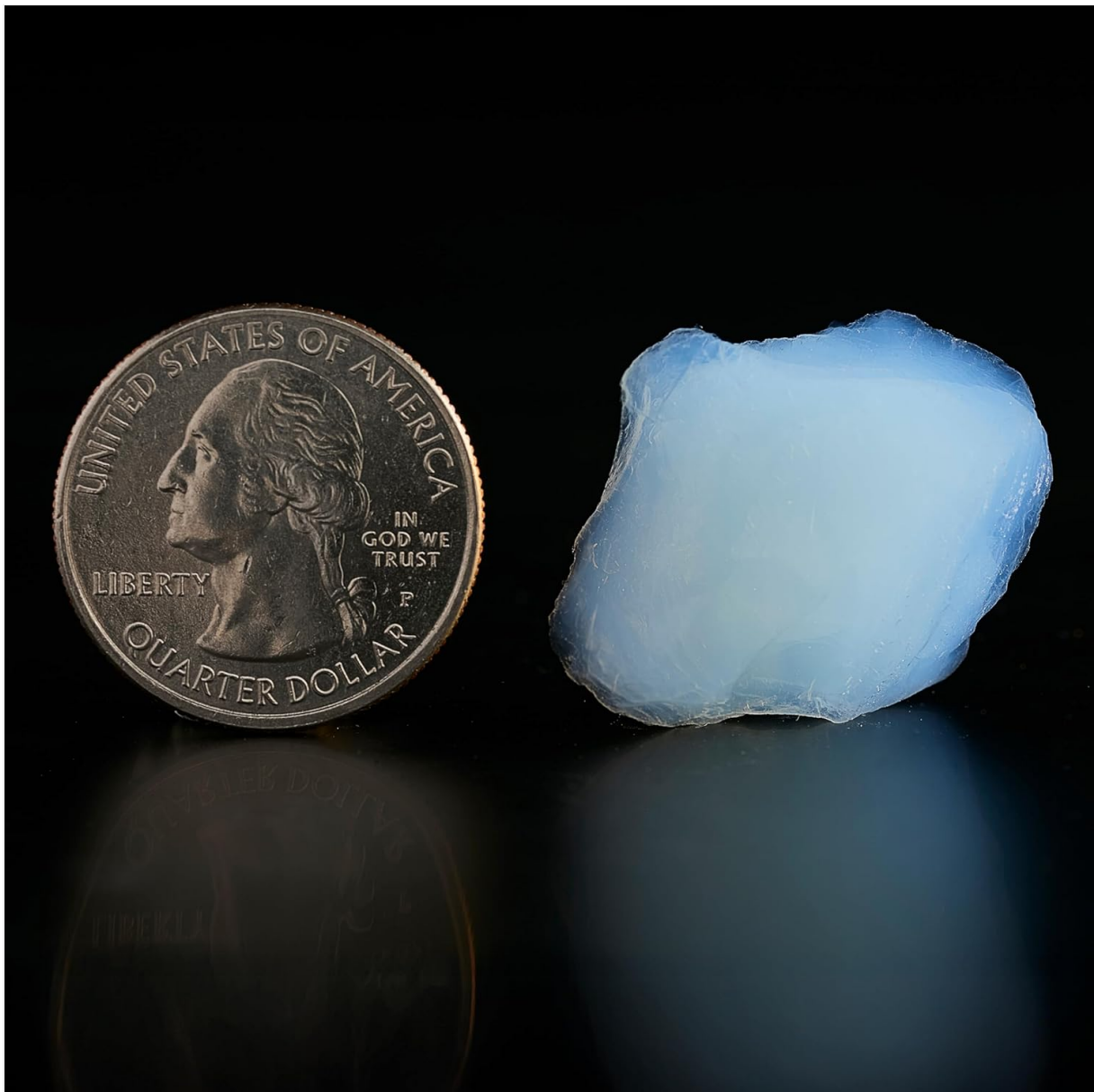
Image 3.1: A silica aerogel chunk displayed next to a US quarter for size comparison.
