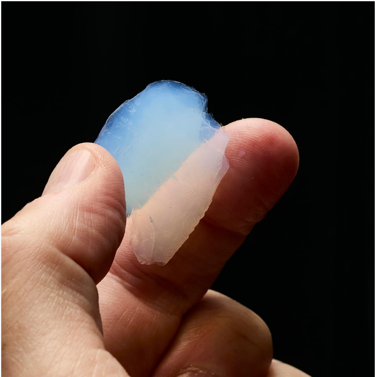
Image 1.1: A piece of silica aerogel held between fingers, showcasing its semi-transparent nature.
