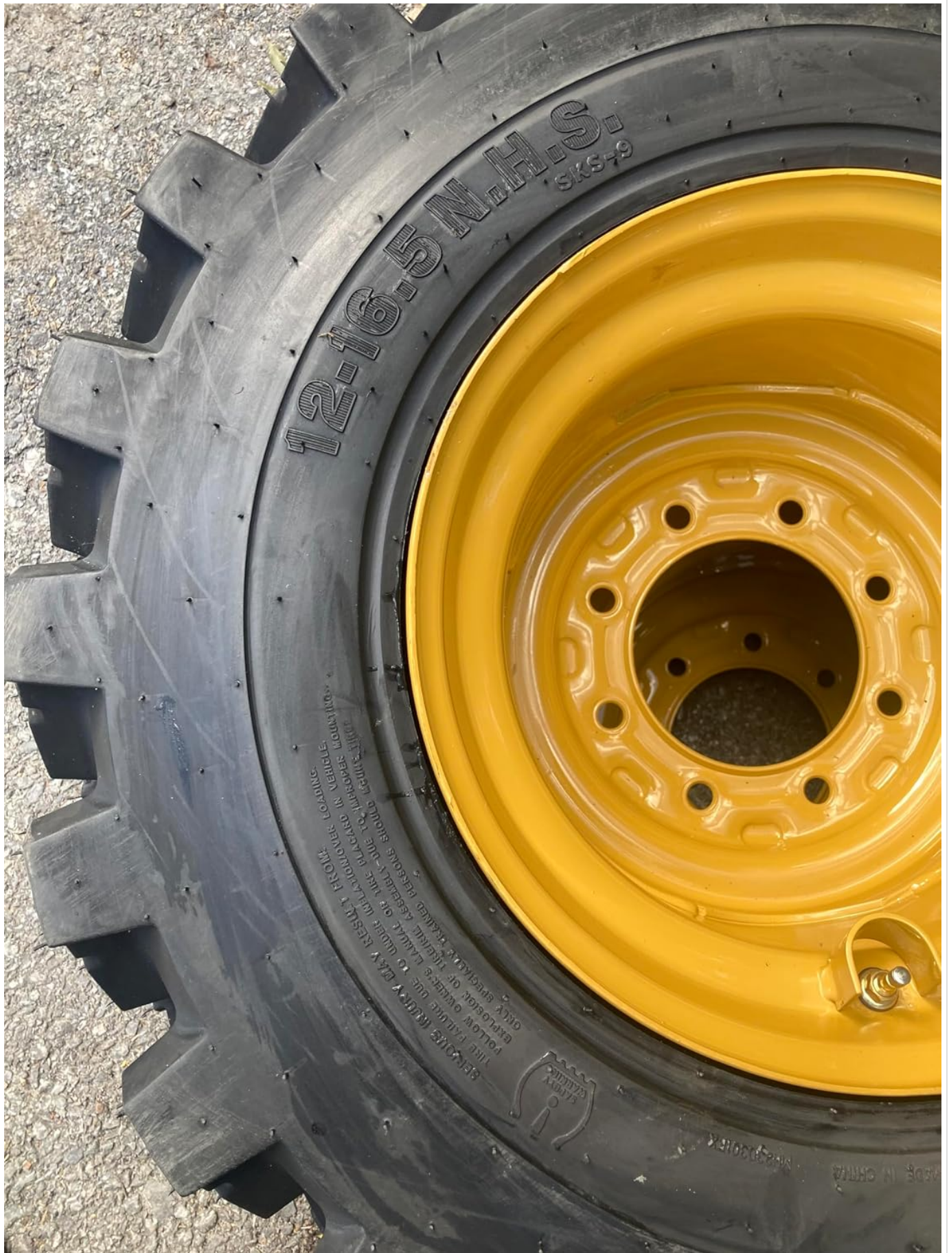
Image: A close-up view of the sidewall of a Forerunner SKS-9 skid steer tire, showing the tire size "12-16.5" and model "SKS-9" clearly visible.
