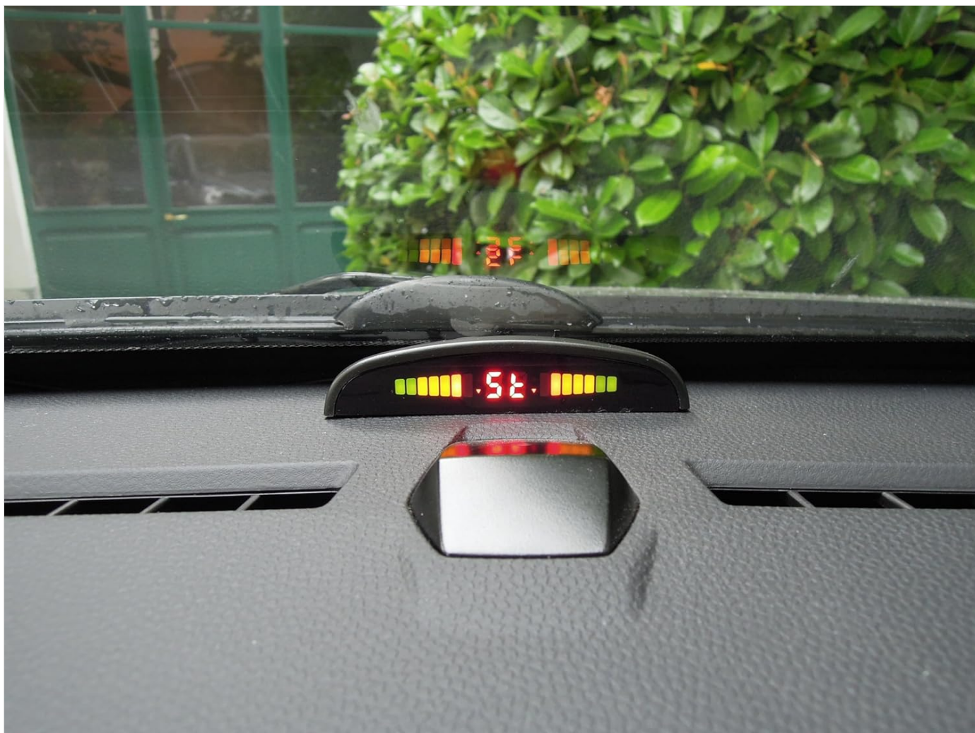
Image: Close-up of the display unit, showing distance reading and proximity bars. Dimensions are 10 cm wide and 2 cm high.
