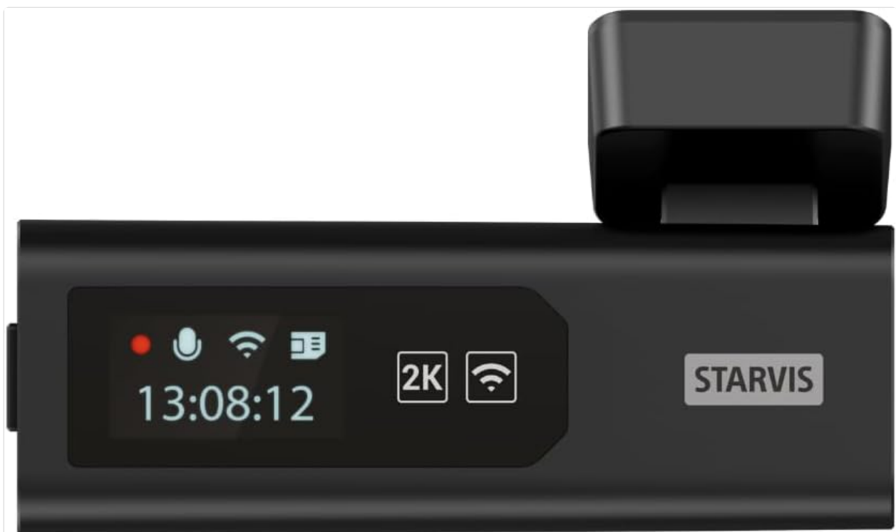
Figure 2.2: Close-up of the Navitel R67 2K's TFT information display, indicating recording status, microphone activity, Wi-Fi connection, 2K resolution, and current time.
