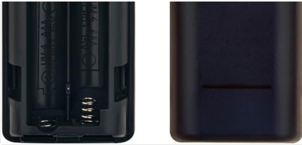
Image: Back of the remote control with the battery compartment open, illustrating where to insert AAA batteries.
