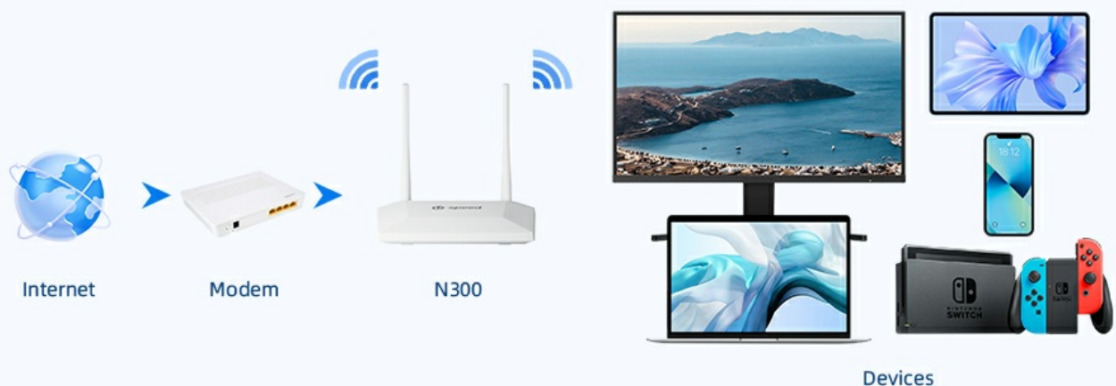
Figure 4.1: Basic Network Connection Diagram
