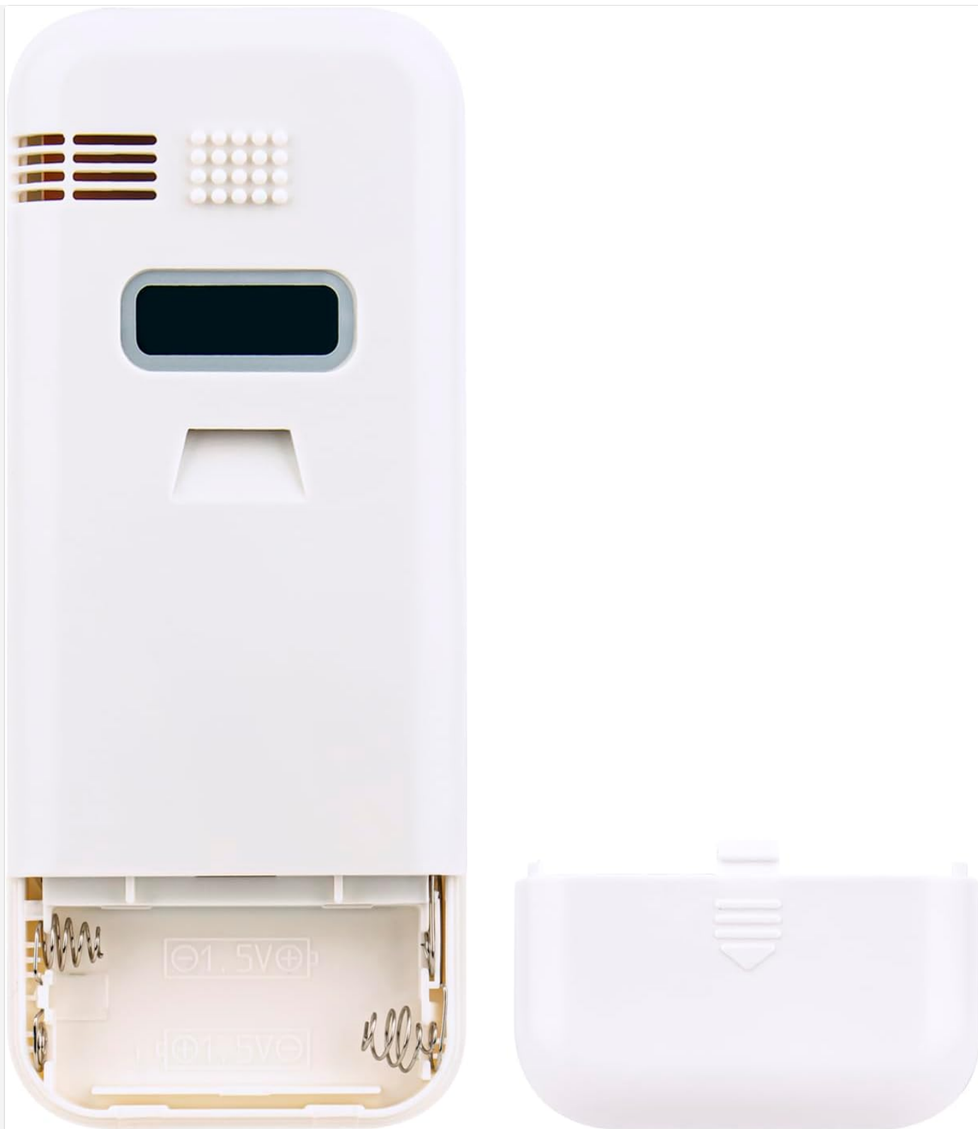
Figure 2.1: Back of the remote control with the battery compartment open, illustrating correct battery placement.
